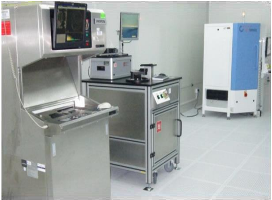
Surface Defect Test: KLA-Tencor製 Surfscan6220 Sheet Resistance Test: Leighton製 LEI-1510-RP非接触測定システム Thickness & Composition Test : Jordan Valley製 QC3 High Resolution X-ray Diffractometer
